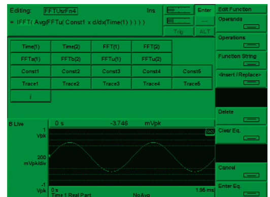
The SR780 doesn't limit you to a few preselected measurements. With user math you can create an infinite variety of measurements.
